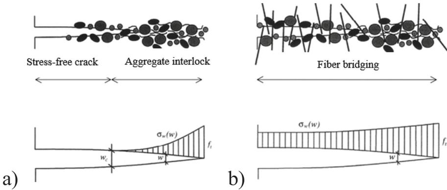
**Fig. 1.** Crack-bridging mechanism, a) in normal concrete and b) in SFRC from [2, 3].
