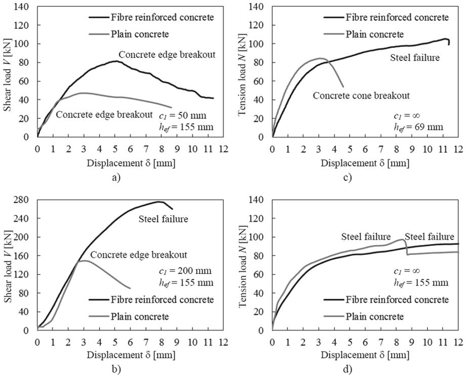
**Fig. 10.** Load-displacement curves of anchor channels-channel bolt-systems cast in plain and fibre reinforced concrete tested in shear with a) small and b) large edge distance and tested in tension with c) small and d) large embedment depth, [6].
