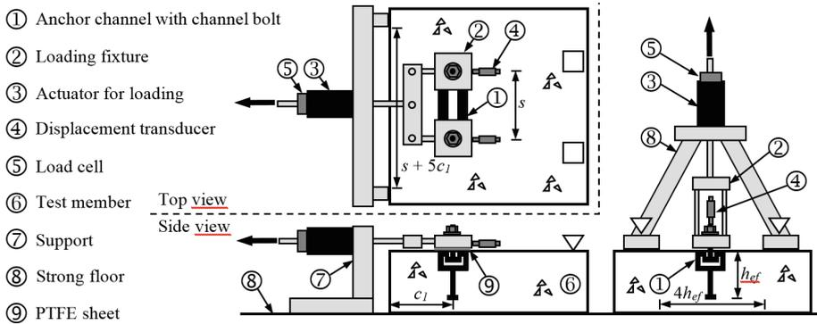
**Fig. 5.** Test setup for shear loading (left) and tension loading (right), [6].
