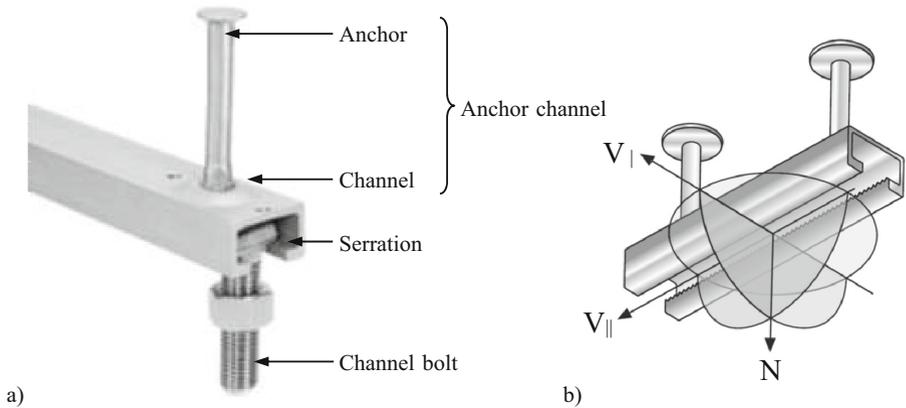
**Fig. 2.** a) Components of anchor channel and channel bolt; b) Serrated systems allow load transfer in all directions.
