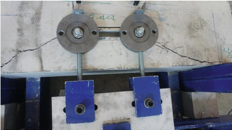
**Fig. 8.** Pictures of the failure under shear loading.
