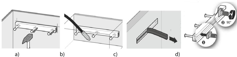
**Fig. 3.** Installation sequence a) attaching of anchor channel to formwork, b) pouring of concrete, c) removing of filler, d) twisting-in of channel bolt.
