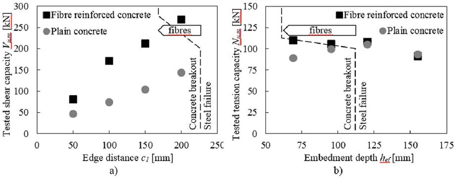
**Fig. 9.** Capacities of anchor channels-channel bolt-systems cast in plain and fibre reinforced concrete tested a) in shear and b) in tension for different edge distances and embedment depths, respectively, [6].
