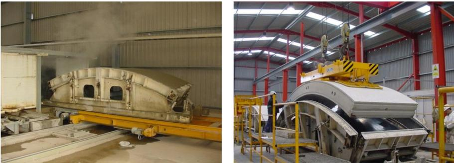
**Fig. 4.** Construction of the tunnel lining segments, from [14].
