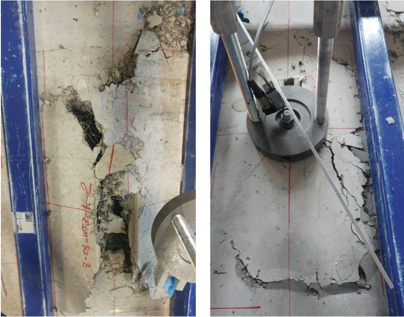
**Fig. 7.** Pictures of the failure under tension loading.
