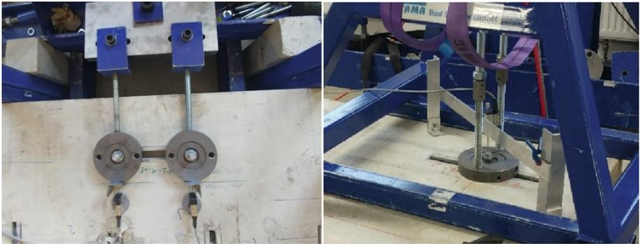
**Fig. 6.** Pictures of the test setup for shear loading (left) and tension loading (right).
