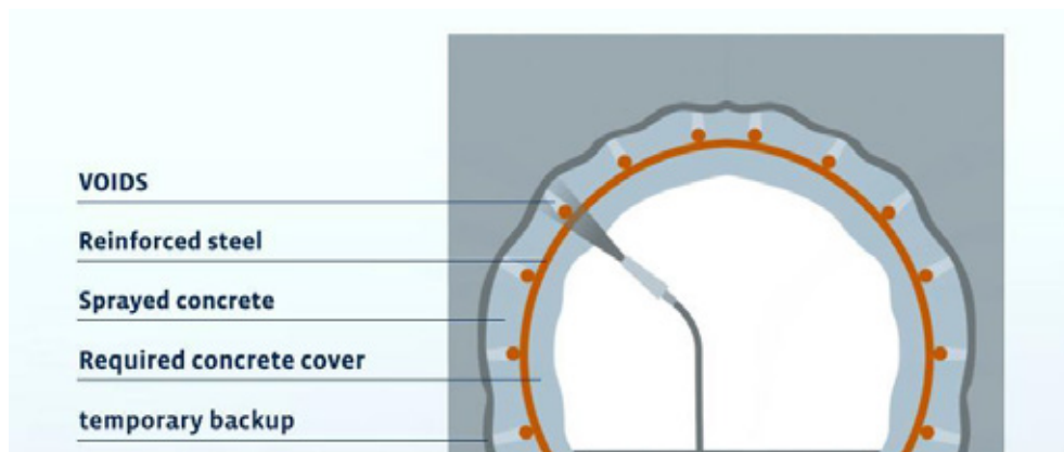
Figure 2 - Solution with conventional reinforced sprayed concrete [3]
