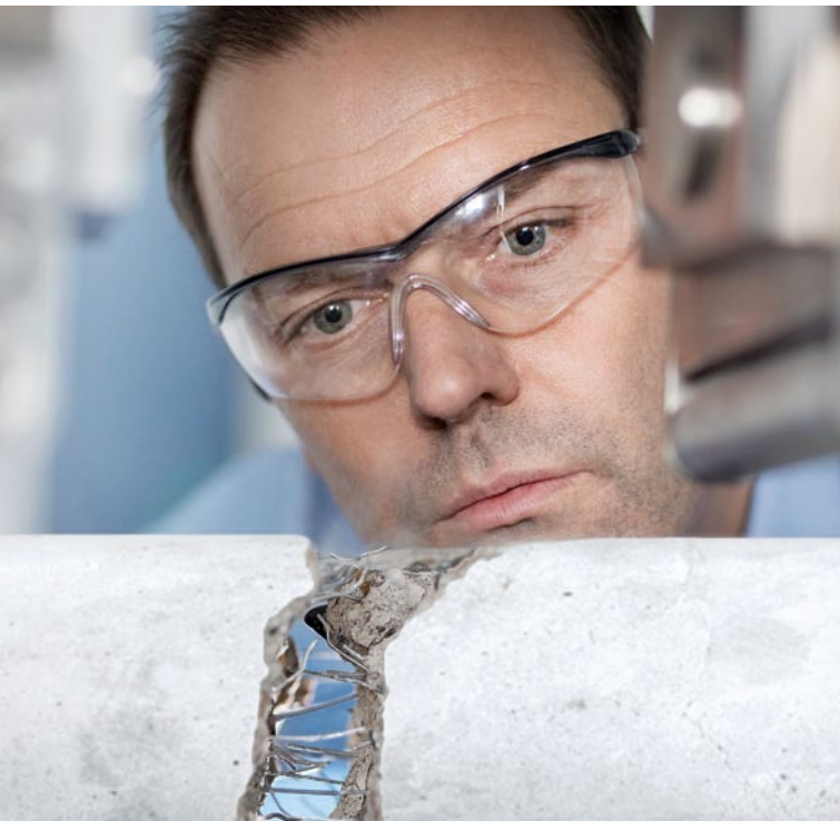
KrampeHarex internal quality control, beam test for SFRC performance
