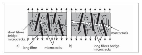
Figure 2: The main principle of hybrid fibre concrete: a) The influence of short thin fibres on the bridging of micro-cracks and the increase of tensile strength; b) the influence of long thick fibres on the bridging of macro-cracks and the increase of ductility (Markovic 2006).
