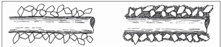
Figure 1: Fine fibre embedded in cement paste (left) and UHPC paste (right). The mechanical fixation of the short and thin fibre is greatly increased by incorporating the ultra-fine particles in the spaces between the cement particles (Hans Henrik Bache 1978).
