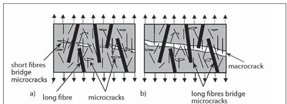
Figure 2: The main principle of hybrid fibre concrete: a) The influence of short thin fibres on the bridging of micro-cracks and the increase of tensile strength; b) the influence of long thick fibres on the bridging of macro-cracks and the increase of ductility (Markovic 2006).
